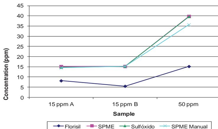
FIGURE 6. Extraction Method Comparison for PCB in transformer oil.
