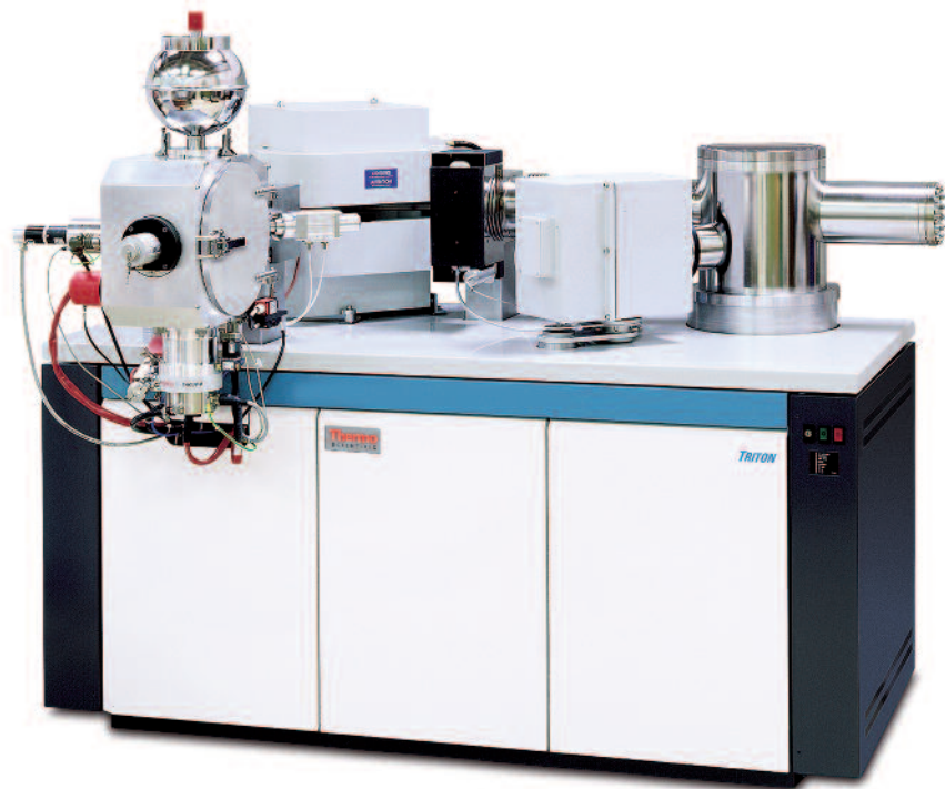
Thermo Scientific TRITON Thermal Ionization Mass Spectrometer
