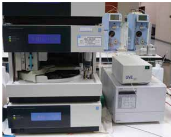
Placement of UVE next to the UltiMate™ 3000 system.
