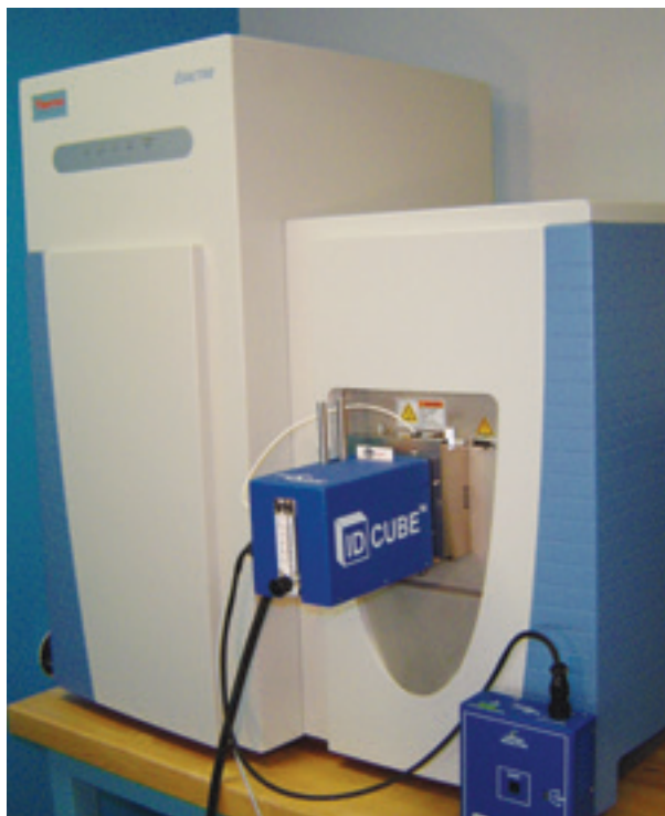
Figure 1. ID-CUBE direct analysis in real time (DART) ionization source coupled with an Exactive MS
