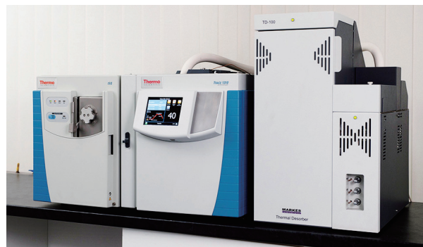
Fig. 1. Automated thermal desorption system with GC-MS detection for VDA 278 analysis, comprised of a Thermo Scientific TRACE 1310 GC, a Thermo Scientific ISQ LT single Quadrupole MS and a Markes TD100 Thermal Desorber
