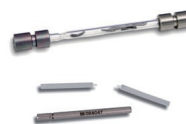
Fig.2. Thermal desorption glass tubes used for VDA 278 analysis with a prepared sample.
