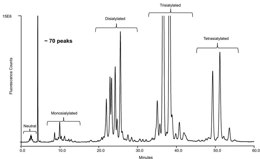
Figure 3: Separation of 2AB-labeled *N*-linked glycans from bovine fetuin by charge, isomerism and size using a binary gradient without acetonitrile on a GlycanPac AXR-1 column
