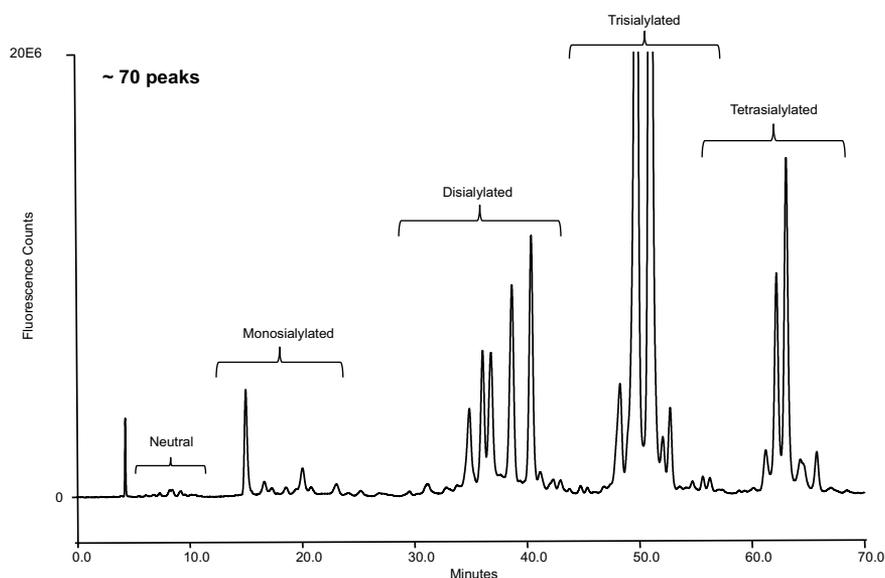
Figure 1: Separation of 2AA-labeled *N*-linked glycans from bovine fetuin by charge, isomerism and size using a ternary gradient with late introduction of acetonitrile on a GlycanPac AXR-1 column
