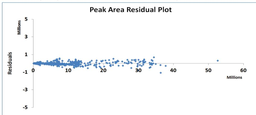
**FIGURE 5. Residual Plot of 410 Calculations of Analyte Concentrations from 41 Donor Samples (  $Y = 0.0593 + 0.9993 X$  R2 = 0.9986 )**
