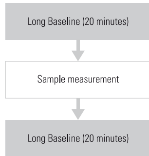
Figure 3: Electrical baselines of amplifiers are determined before and after the analysis to get most accurate readings ( < 1 \mu\text{V} ).
