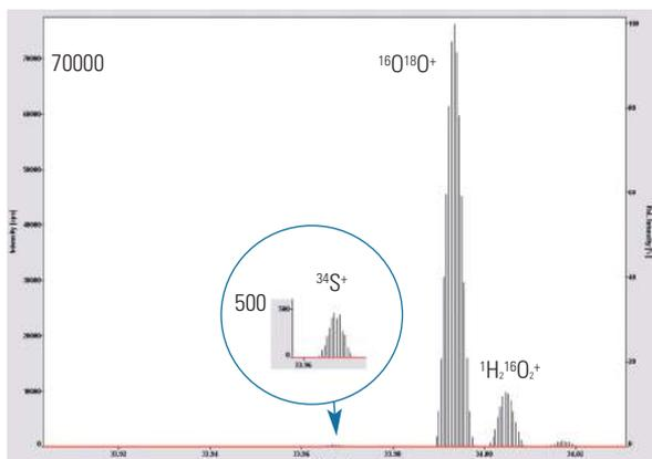
Figure 4:  $^{34}\text{S}$  interferences in acetonitrile.
