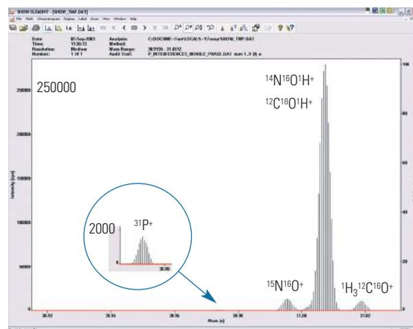
Figure 2: Phosphorus interferences in 4 mmol L<sup>-1</sup> ammonium acetate and 2% methanol.
