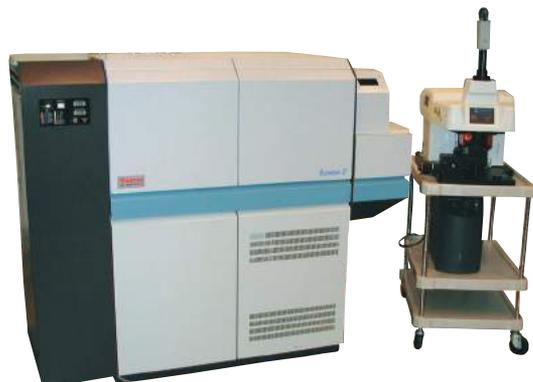
Figure 3: Thermo Scientific ELEMENT 2 with New Wave UP213 laser system.
