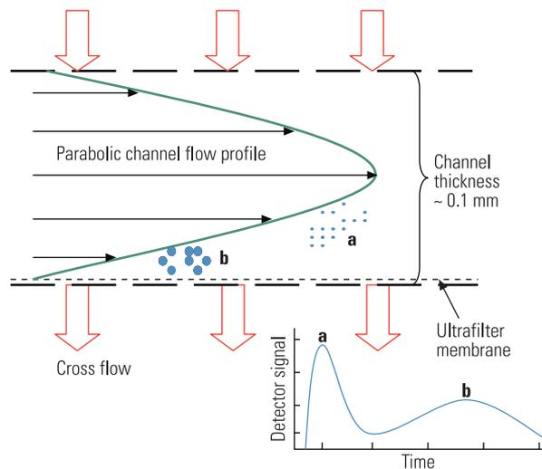
Figure 7: Flow Field-Flow Fractionation Principle.
