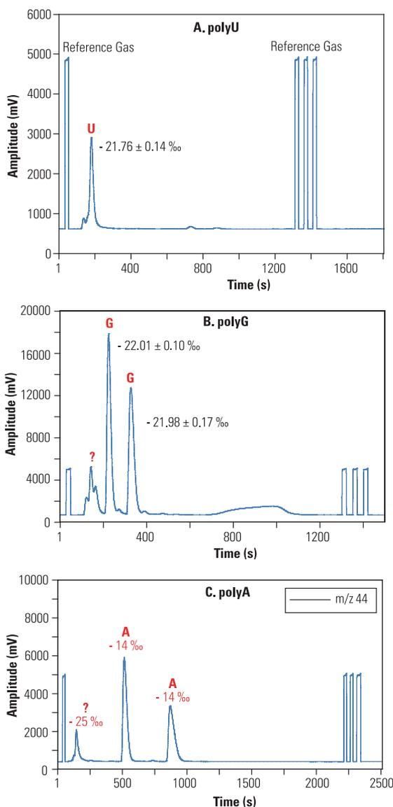
Figure 2: *irm*-LC/MS analysis of NaOH-hydrolyzed polynucleotides. RNA hydrolysis and HPLC separations were done as for the experiments in Figure 1, except that a 2.1 mm diameter column was used. Numbers next to peaks are  $\delta^{13}\text{C}$  (PDB) values.
