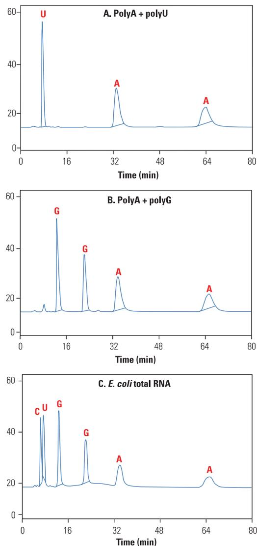
Figure 1: HPLC separation of NaOH-hydrolyzed polynucleotides and RNA. Approximately 4  $\mu\text{g}$  of RNA were digested to mononucleotides by 15 min incubation at 50  $^{\circ}\text{C}$  in 0.2 N NaOH, and separated by HPLC as described in the Experimental section.
