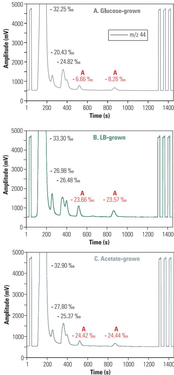
Figure 3: *irm*-LC/MS analysis of NaOH-hydrolyzed *E. coli* RNA. RNA was extracted from overnight cultures of *E. coli* grown on LB medium, or on M9 minimal salts with glucose or acetate as sole carbon source<sup>[6]</sup>; denatured in 0.2 N NaOH; separated by HPLC on a 2.1 mm diameter HyPURITY AQUASTAR column; and introduced to the IRMS via the LC IsoLink interface.  $\delta^{13}\text{C}$  values are the average of three determinations; errors were < 1 ‰ and are shown in Figure 4.
