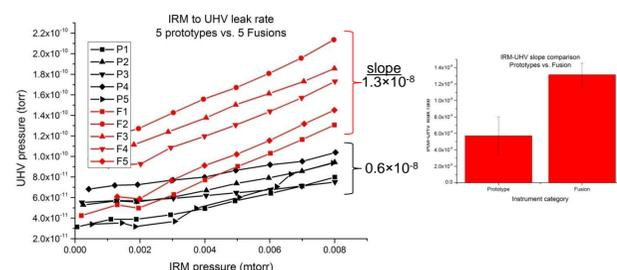
**FIGURE 2.** IRM to UHV leak rates, prototypes with vacuum modifications compared with Orbitrap Fusion systems. Higher base pressure in Orbitrap Fusion systems is due to initial system pumpdown.
