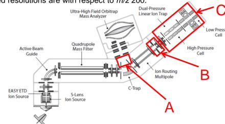
**FIGURE 1.** Modified Orbitrap Fusion mass spectrometer, with areas of modification: A, material removed to allow better gas conductance; B, nitrogen gas allowed to pass into dual linear trap chamber; and C, increased pumping capacity from 80 l/s to 290 l/s to handle the increased gas load from (B).
