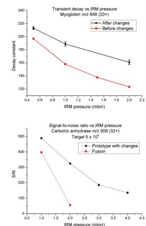
**FIGURE 3.** (top) Transient decay versus IRM pressure, on the same instrument before and after the changes. Decay is faster (smaller time constant) at higher pressures prior to the changes. Myoglobin 20+ is used because isolating this charge state results in a transient comprised of 8 beats. Therefore at higher pressures where fewer beats are visible, decay can still be accurately measured.
