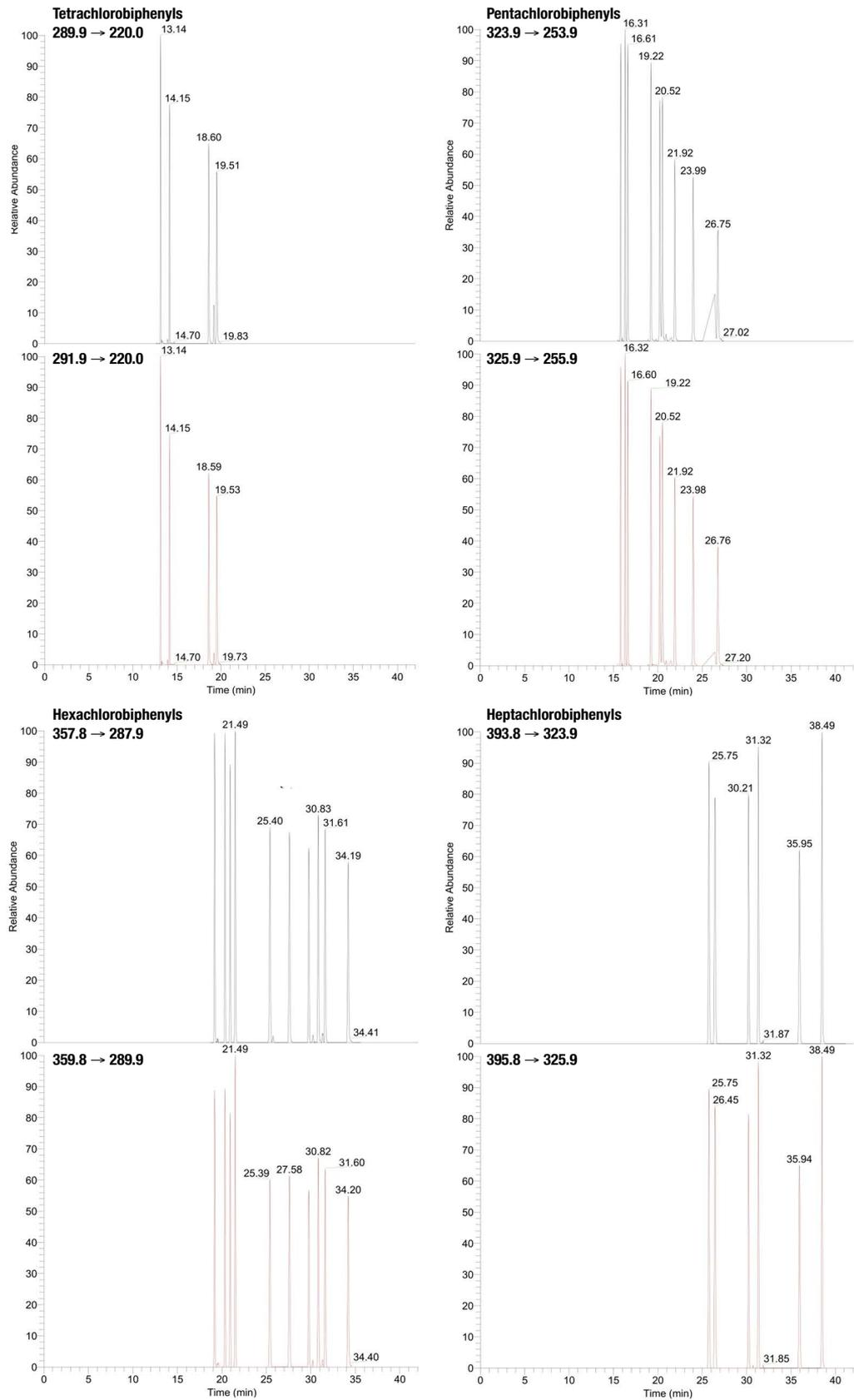
Figure 5. SRM chromatograms for a 5 µg/kg PCB-spiked soil sample after ASE-extraction and concentration.
