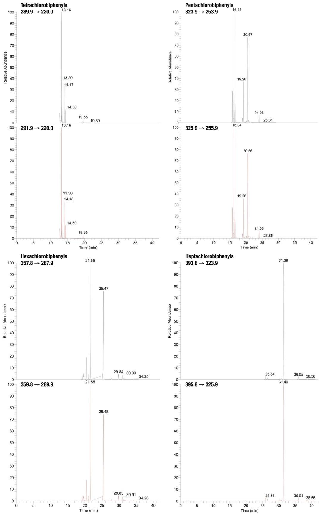
Figure 7. PCB SRM chromatograms for a contaminated soil sample.
