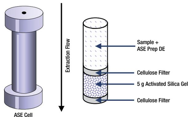
Figure 3. Extraction cell schematic.
