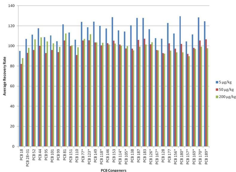
Figure 4. Average recovery rates for the 5, 50, and 200 µg/kg spike levels.
