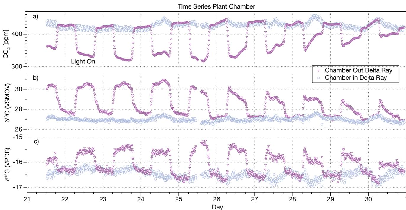
Figure 4. a) Time series of CO<sub>2</sub> concentration of Delta Ray chamber in and chamber out; b) time series of δ<sup>18</sup>O of the Delta Ray IRIS of plant chamber in and out; c) δ<sup>13</sup>C of the Delta Ray IRIS of plant chamber in and out
