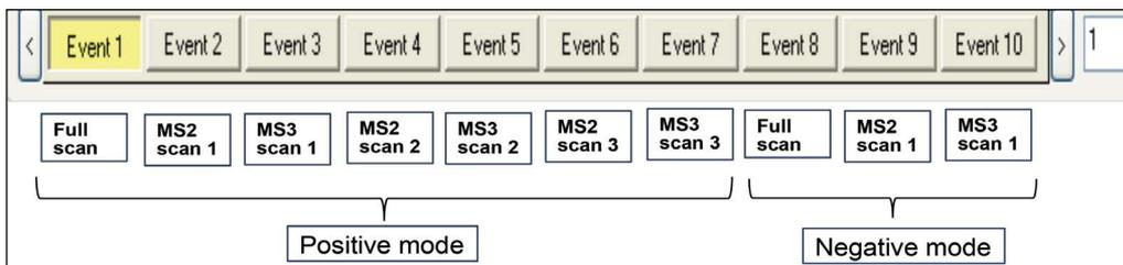
Figure 5. LTQ method scan events: A positive ion full-scan event is followed by MS2 (and associated MS3) scan events for the three most abundant compounds from a targeted list. This is repeated in negative ionization mode with the single most abundant targeted compound.
