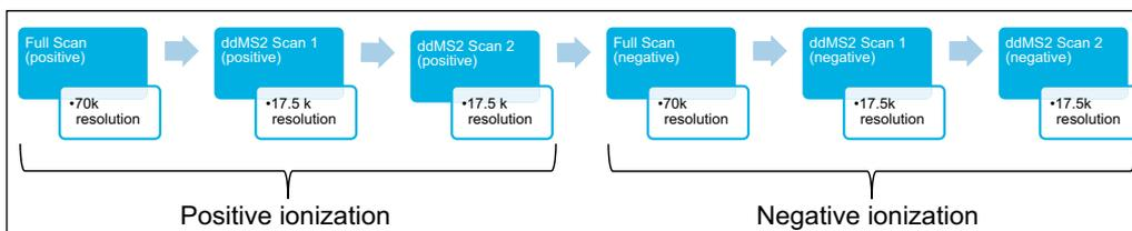
Figure 6. Q Exactive Focus MS method scan events: After a full-scan event in positive ionization mode, two ddMS2 scan events are triggered for the two most abundant masses from a targeted inclusion list. This is then repeated in negative ionization mode.
