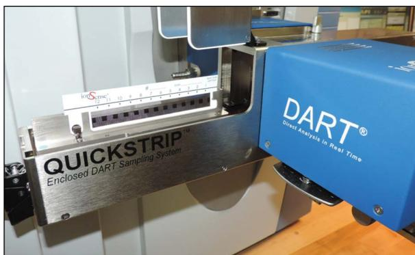
Figure 3. DART QuickStrip direct injection source.
