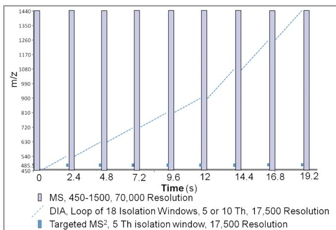
**Figure 3.** Pictorial representation of extending the capabilities of pSMART for mixed mode quantitation. The original pSMART method is represented by MS acquisition with one targeted PRM event with the idea to stratify which peptides can be quantified by MS and which ones may need the added sensitivity of PRM. (Koomen, 2015).
