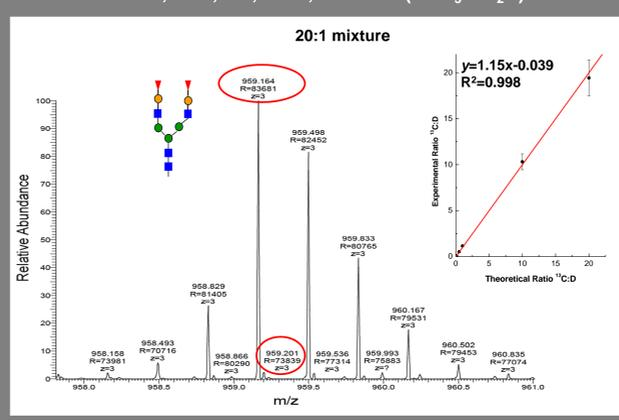
FIGURE 4. HCD QUIBL quantification of the fetuin tetra-sialylated glycan using sialic acid fragment ion at *m/z* 382. Orbitrap spectra were acquired at 100K RP. Inset shows correlation between the theoretical and experimental ratios for mixtures at 20:1, 10:1, 1:1, and 0.5:1 (<sup>13</sup>CH<sub>3</sub>:CH<sub>2</sub>D).
