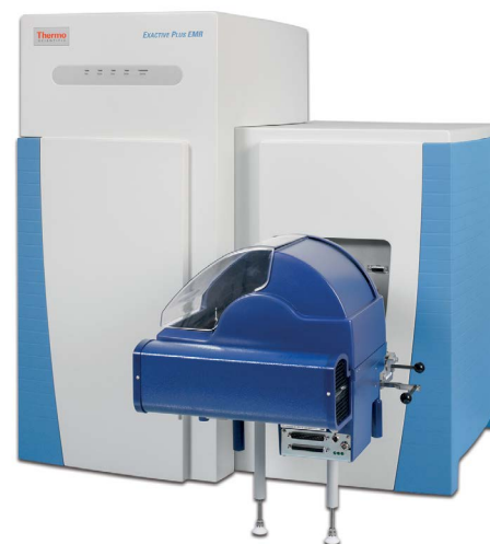
Figure 1. Exactive Plus EMR mass spectrometer equipped with a TriVersa NanoMate chip-based electrospray ionization interface
