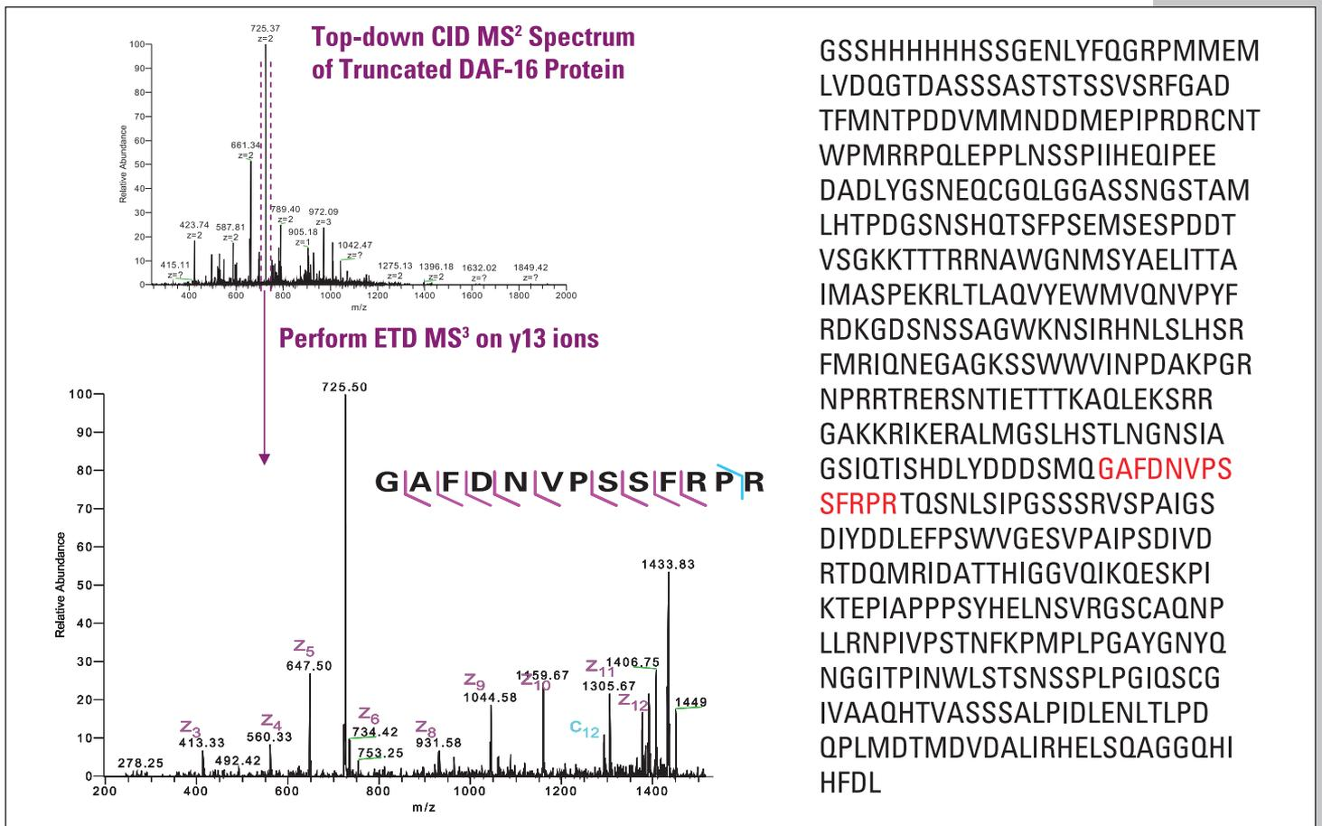
Figure 6: Identification and complete sequencing of C-terminus using ETD MS<sup>3</sup> of y13 ions
