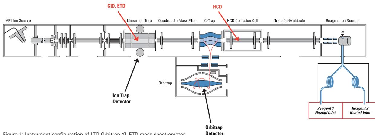
Figure 1: Instrument configuration of LTQ Orbitrap XL ETD mass spectrometer
