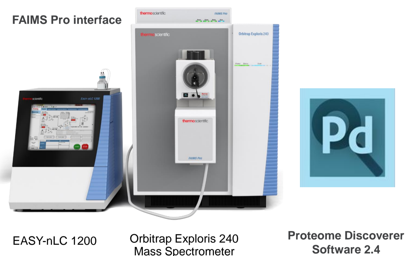
Figure 1. LC-MS setup for cross laboratory performance evaluation and HeLa curve Study.
