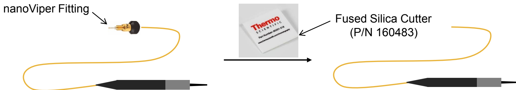
Approach to customize the transfer line length of EASY-Spray emitter
