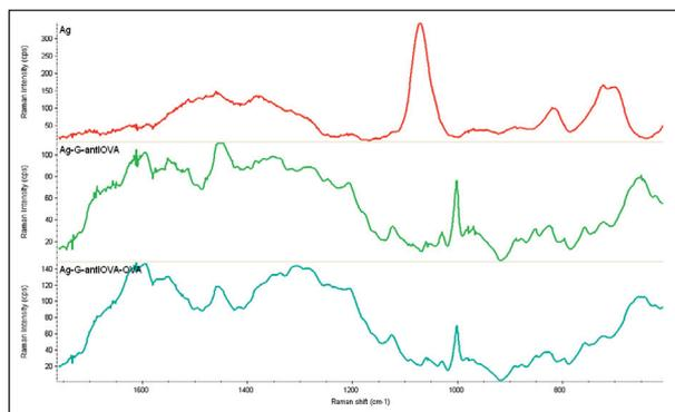
Figure 2a: Average spectra of the bare silver dendrite, silver dendrite with protein G and antiOVA bound to it (Ag-G-antiOVA), and silver dendrite with protein G and antiOVA with OVA captured (Ag-G-antiOVA-OVA)
