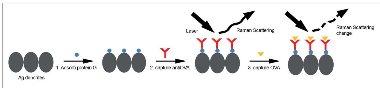
Figure 1: The preparation of the modified silver dendrites and Surface-Enhanced Raman Scattering (SERS) analysis of the bound protein
