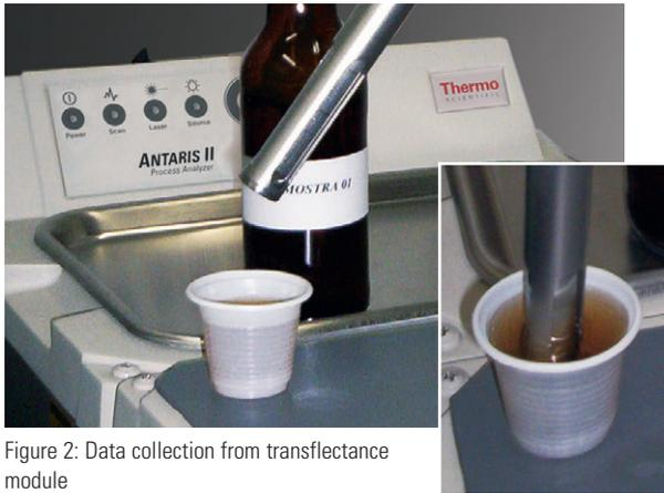
Figure 2: Data collection from transreflectance module
